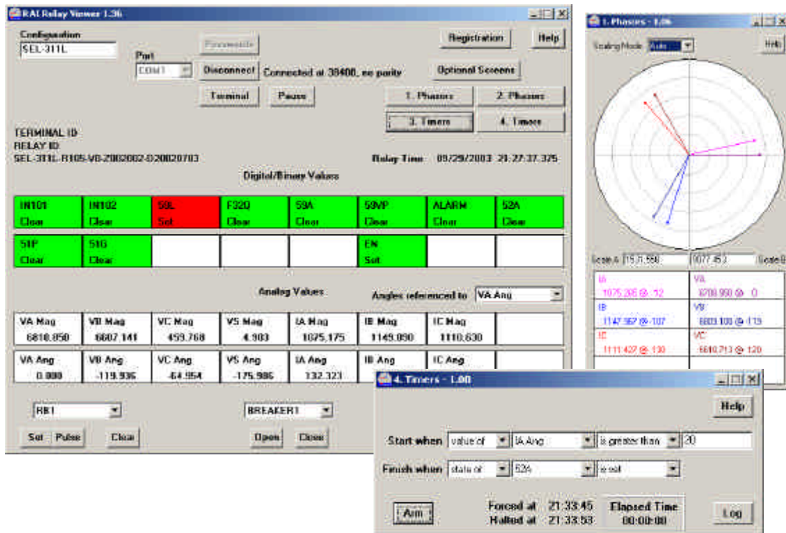
Figure 9: Example Third-party Relay Monitoring Software Showing Digital Logic States, Metering Phasors, and Test Timing Records
